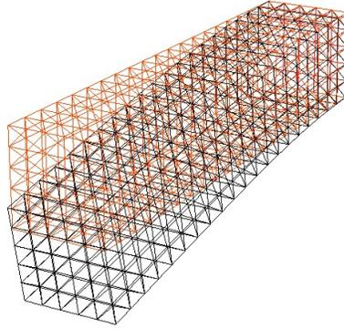
Fig. 5.10: 3d Beam deformed and undeformed box
